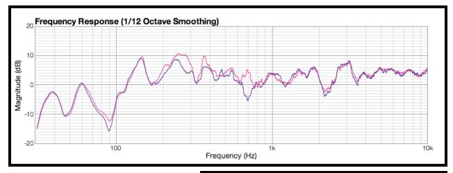
The significant dip at 90 Hz is a result of a couple issue – a Tangential Mode at 90.1 Hz and a side-to-side Axial Mode at 90.4 Hz. Thicker corner traps will help the Tangential issue and thicker side wall panels will improve the the Axial Mode issue.
